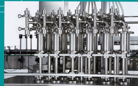
Precision concentrated heavy-walled SS316 cylinders
